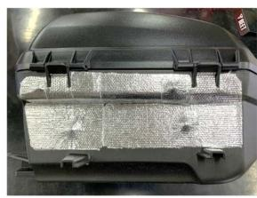
With a heat insulating sheet attached
