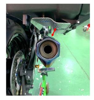
With the heat shield attached If you put your luggage in the pannier case, it will hang down due to its weight, so please secure a clearance of about the red arrow.
